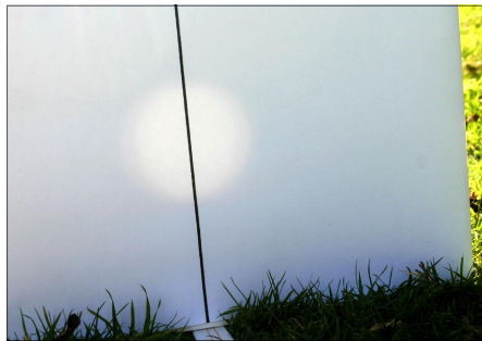
Fig. 5. The image of the sun from the front silvered version with the reflecting area reduced to a 'pinhole' of 1.5 cm square.
