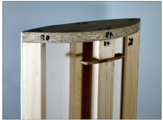
Fig. 3 (above). Interior of a soundbox, showing support for bridge
