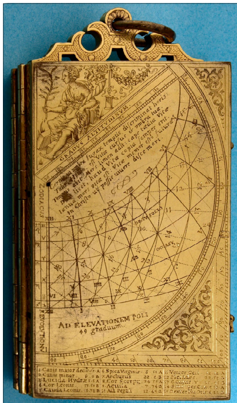
Fig. 4. The folded horizontal stereographic projection on the outside of J.A. Linden's 1596 compendium. Courtesy of the Trustees of the British Museum.
