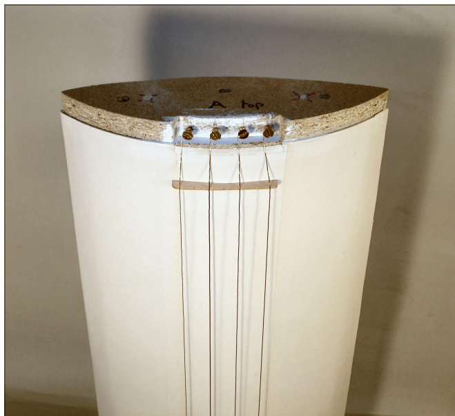
Fig.5. Soundbox with tensioned brass strings.
